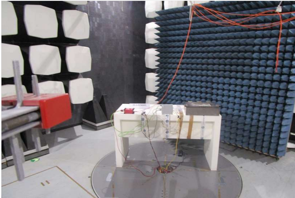
Photograph 3: EUT test setup in the semi anechoic chamber, overview
