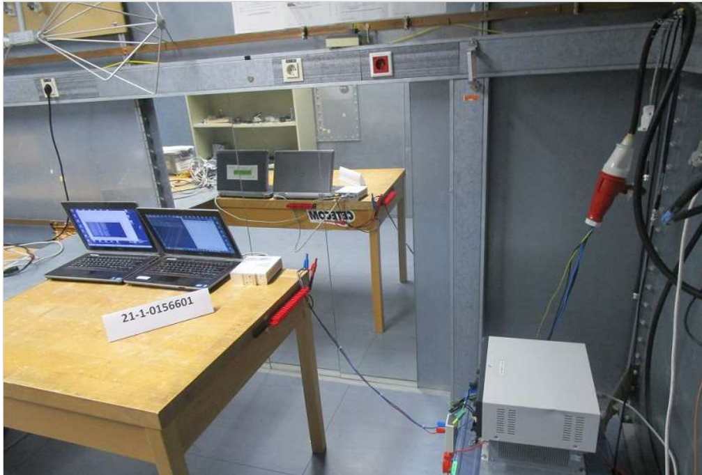
Photograph 1: EUT test setup Conducted emissions on DC-Power lines
