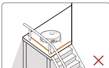
④ If the Robot is used in a suspended environment or a dangerous area such as a fireplace or an exhaust port, please use a solid physical barrier to prevent the robot from accidentally falling or entering to cause personal or property damage, and do not use a magnetic boundary strip for isolation.
