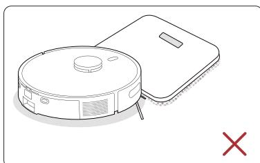
③ The Robot may climb onto objects less than 20mm in height. If possible, remove these objects.
