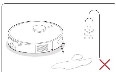
⑤ Make sure the Robot is kept away from wet areas and viscous substances during cleaning.
