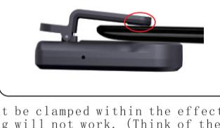
C) The sensor point must be clamped within the effective area of the screen, otherwise, page-turning will not work. (Think of the sensor point as equivalent to a human finger.)
