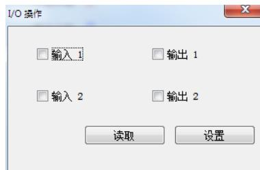
[Input 1/2]: It is the photoelectric input port control, configure the photoelectric input port to be enabled.
