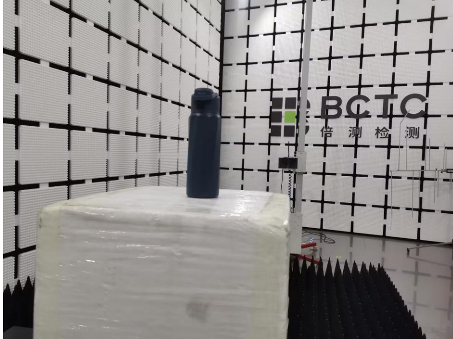
Spurious Emission Test Setup (Above 1GHz)
