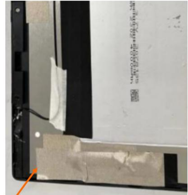
Wiring with conductive cloth
