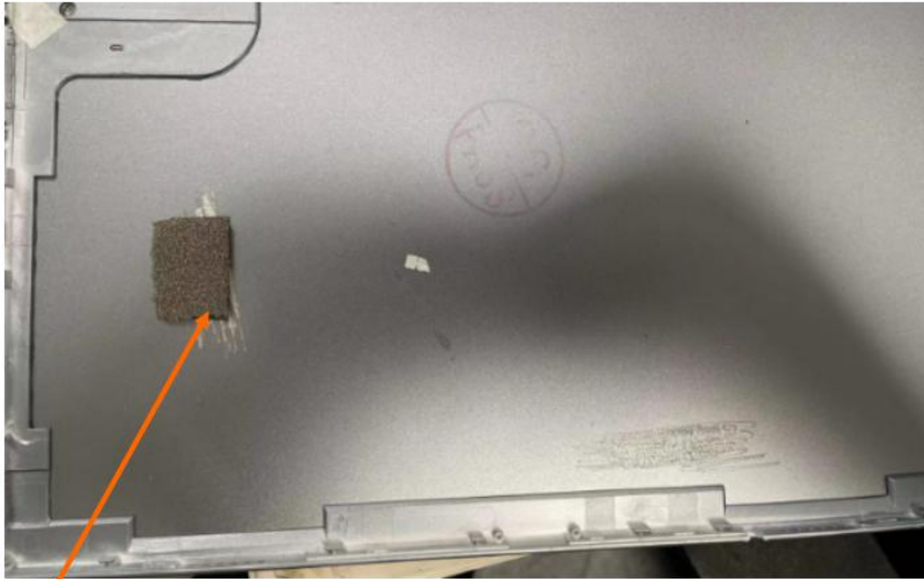
The rear shell is grounded to the mainboard
