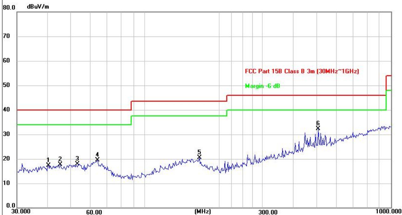
Antennal Polarity& Test Distance: Vertical at 3m
