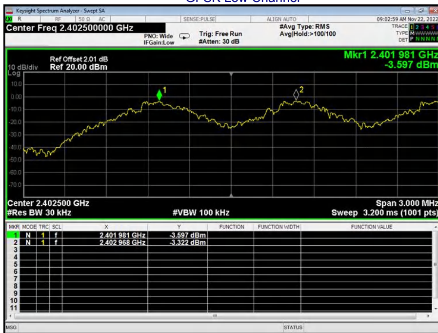
Test plots GFSK Low Channel
