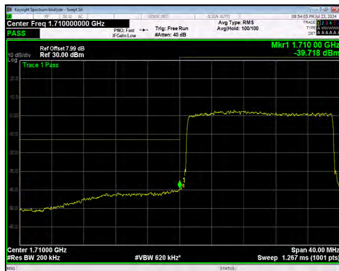
Band4 16QAM BW=20MHz Channel=20300 RB Size=1 Position=#0 Extended
