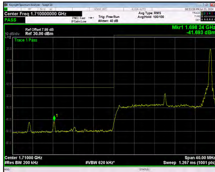
Band4 16QAM BW=20MHz Channel=20050 RB Size=100 Position=#0 Extended
