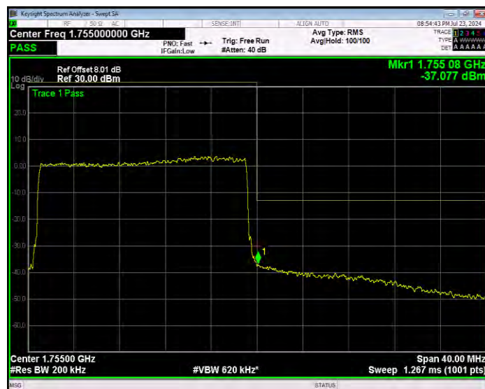
Band4 16QAM BW=3MHz Channel=19965 RB Size=1 Position=#0 Extended
