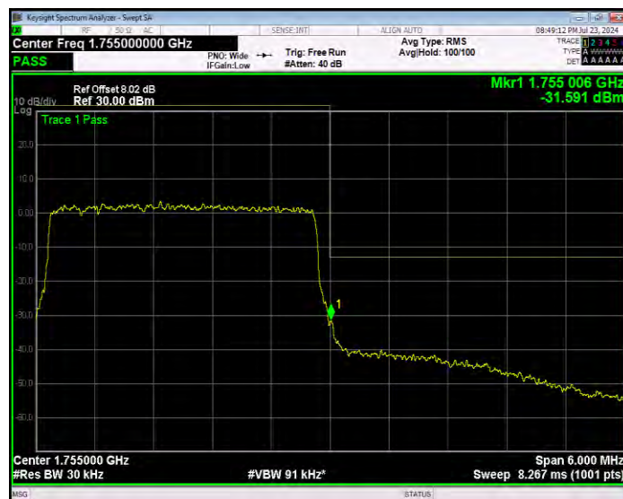
Band4 16QAM BW=5MHz Channel=19975 RB Size=1 Position=#0 Extended
