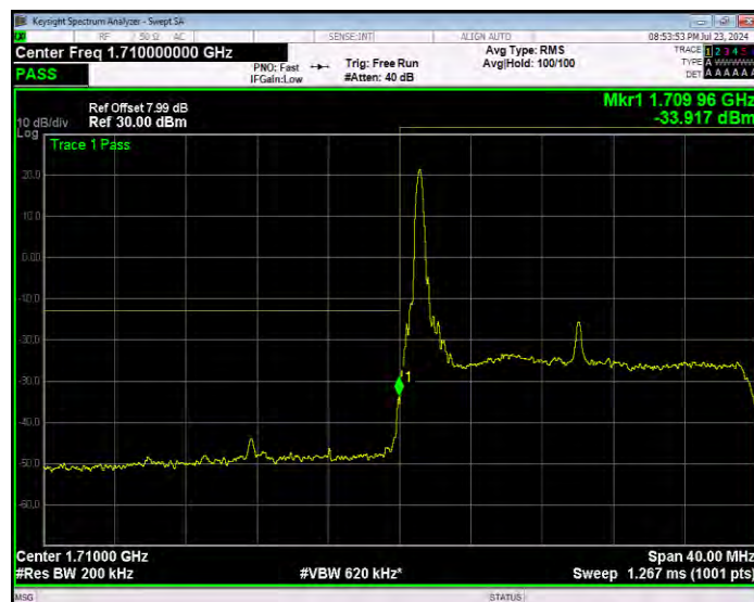
Band4 16QAM BW=20MHz Channel=20050 RB Size=1 Position=#Max Extended
