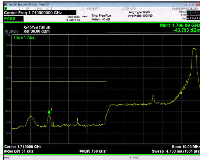
Band4 16QAM BW=5MHz Channel=19975 RB Size=25 Position=#0 Extended
