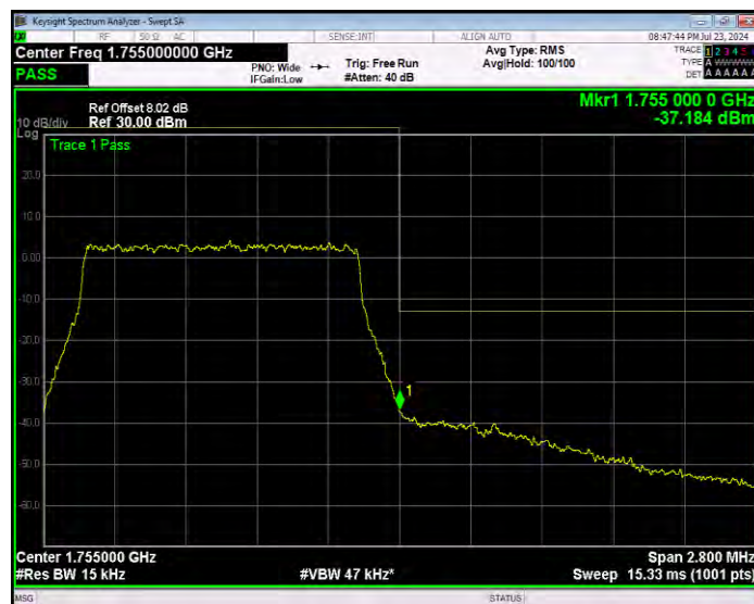
Band4 16QAM BW=10MHz Channel=20000 RB Size=1 Position=#0 Extended
