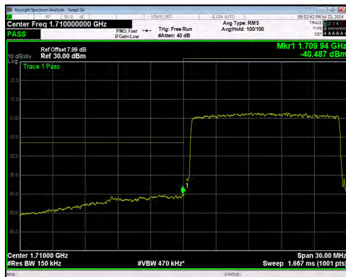
Band4 16QAM BW=15MHz Channel=20325 RB Size=1 Position=#0 Extended
