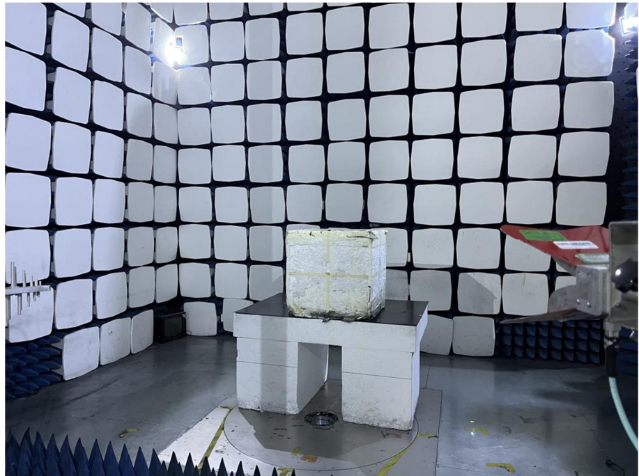
Radiation Emission Test Setup (1GHz to 18GHz)
