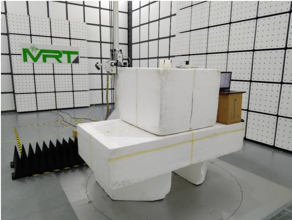
Description: Radiated Emission Test Setup for 9kHz~30MHz
