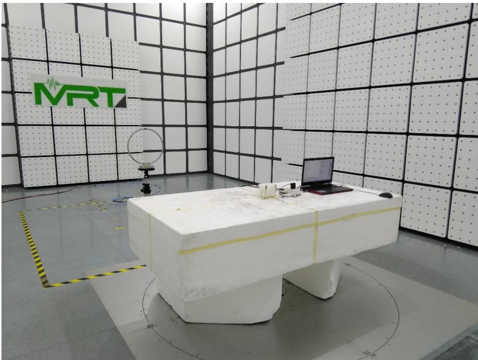
Description: Radiated Emission Test Setup for 9kHz~30MHz
