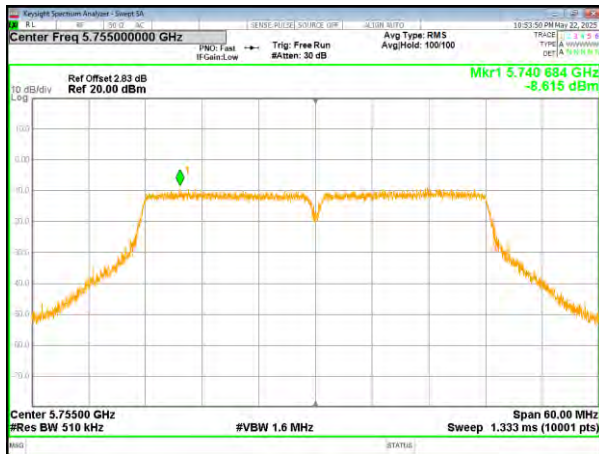
(802.11ac40) PSD plot on channel 159
