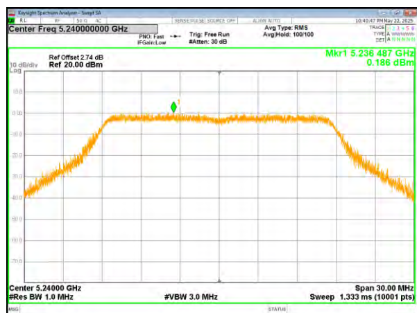
(802.11n20) PSD plot on channel 48
