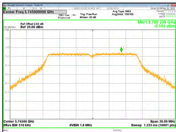
(802.11a) PSD plot on channel 157
