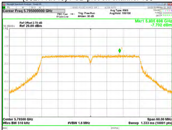
(802.11ac40) PSD plot on channel 159
