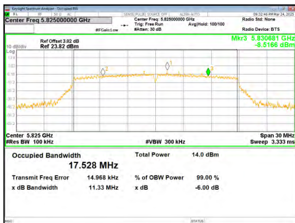
(802.11ac20) plot on channel 165
