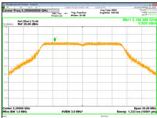
(802.11a) PSD plot on channel 48
