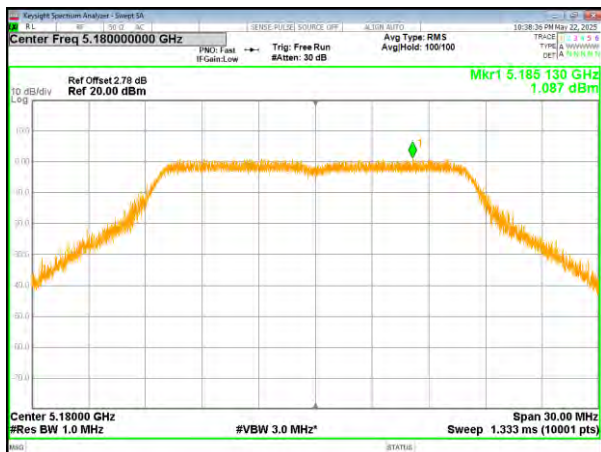
(802.11a) PSD plot on channel 36
