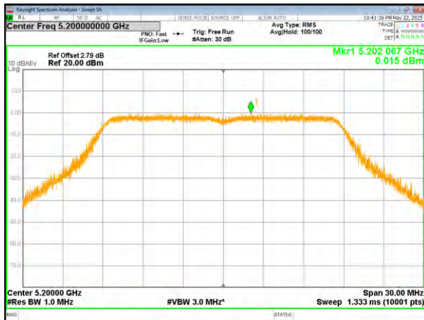
(802.11ac20) PSD plot on channel 48
