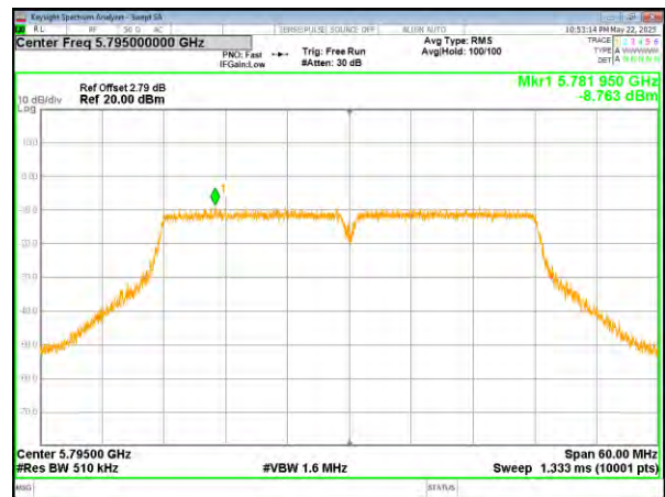
(802.11n40) PSD plot on channel 159
