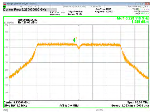
(802.11n40) PSD plot on channel 46
