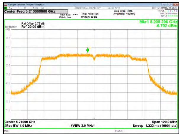
(802.11ac80) PSD plot on channel 42
