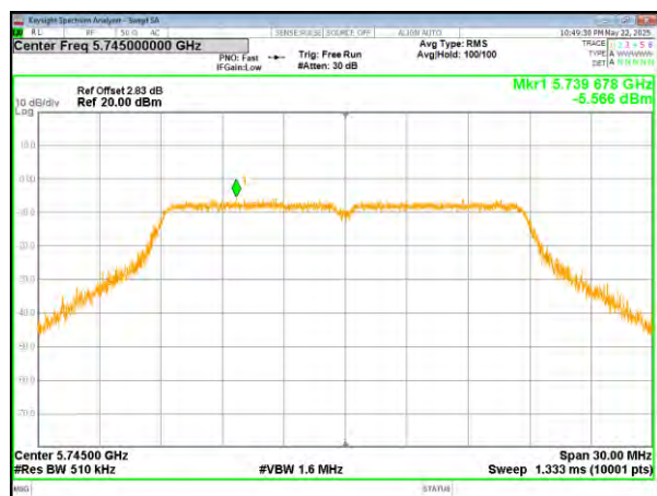
(802.11n20) PSD plot on channel 157
