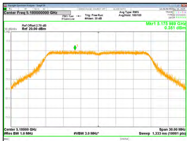
(802.11n20) PSD plot on channel 36
