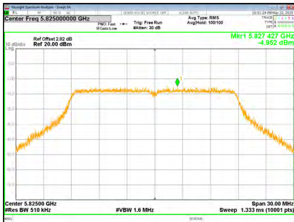
(802.11ac20) PSD plot on channel 165
