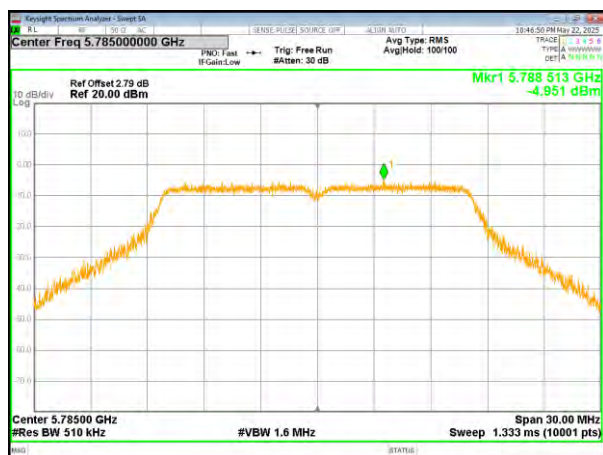
(802.11a) PSD plot on channel 165
