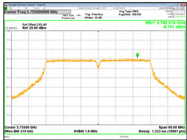
(802.11n40) PSD plot on channel 159
