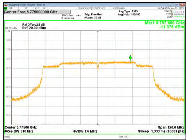
(802.11ac80) PSD plot on channel 155
