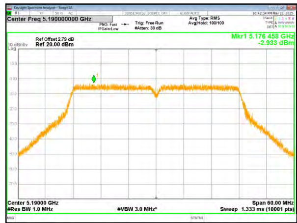
(802.11n40) PSD plot on channel 46
