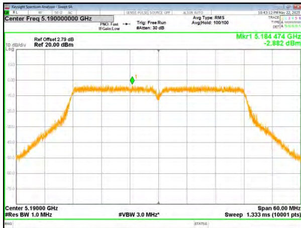
(802.11ac40) PSD plot on channel 46
