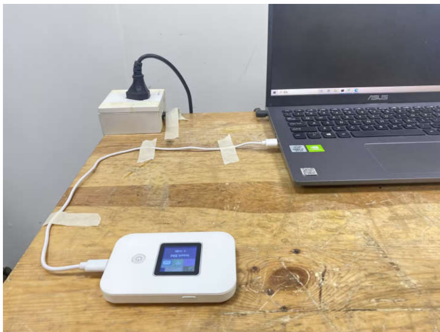
Conducted Emissions Test Setup-2(Close up)
