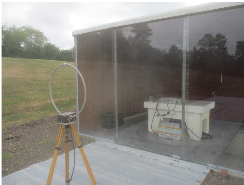
Parallel Antenna Polarization
