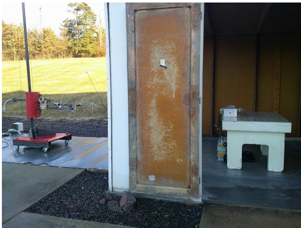
Horizontal Antenna Polarization, 30 to 200 MHz
