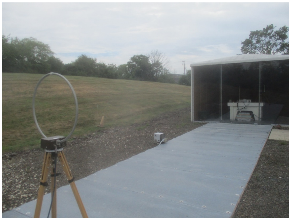
Parallel Antenna Polarization
