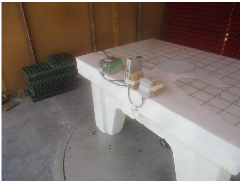
EUT Configuration, 30 MHz to 1 GHz
