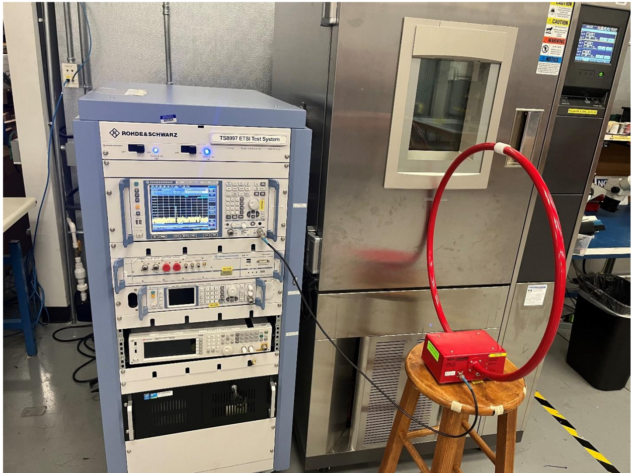
Temperature Chamber / Frequency Stability Tests
