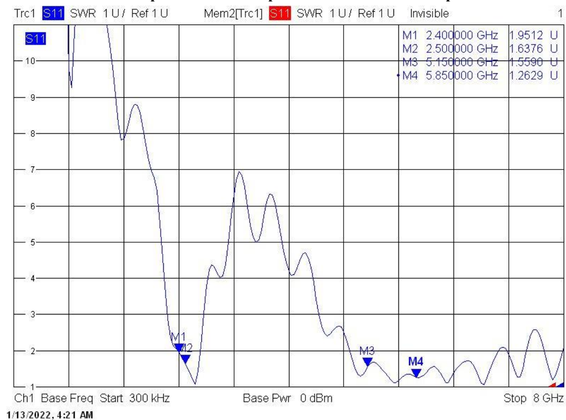
VSWR parameter in sample antenna tested in free space
