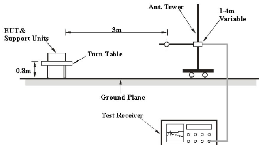
The radiated emission tests were performed in the 3-meter chamber test site, using the setup accordance with the ANSI C63.10-2013.
