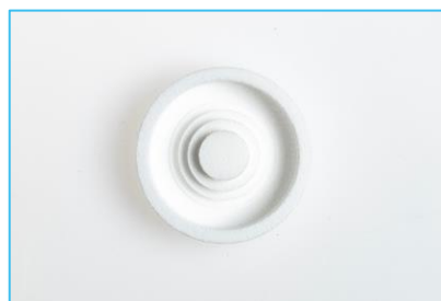
Figure 2.5. FZP lens diameter 36.3 mm and height 7.8 mm
