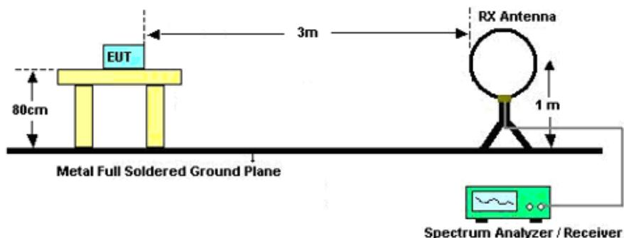
For radiated emissions from 30MHz to 1GHz
