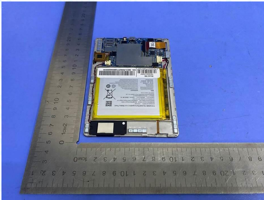
Photo 9 Internal of EUT
