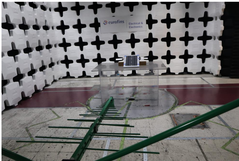
Figure 7. Radiated Spurious Emissions, ISM 900 & BLE (30 MHz – 1 GHz) Test Setup
