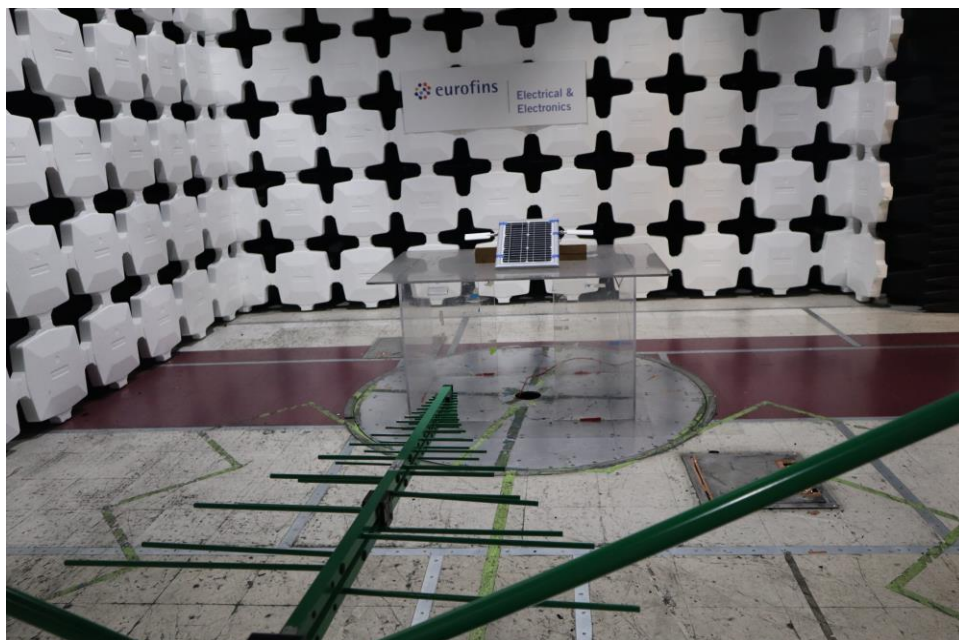
Figure 2. Radiated Spurious Emissions, Idle Mode (30 MHz – 1 GHz) Test Setup
