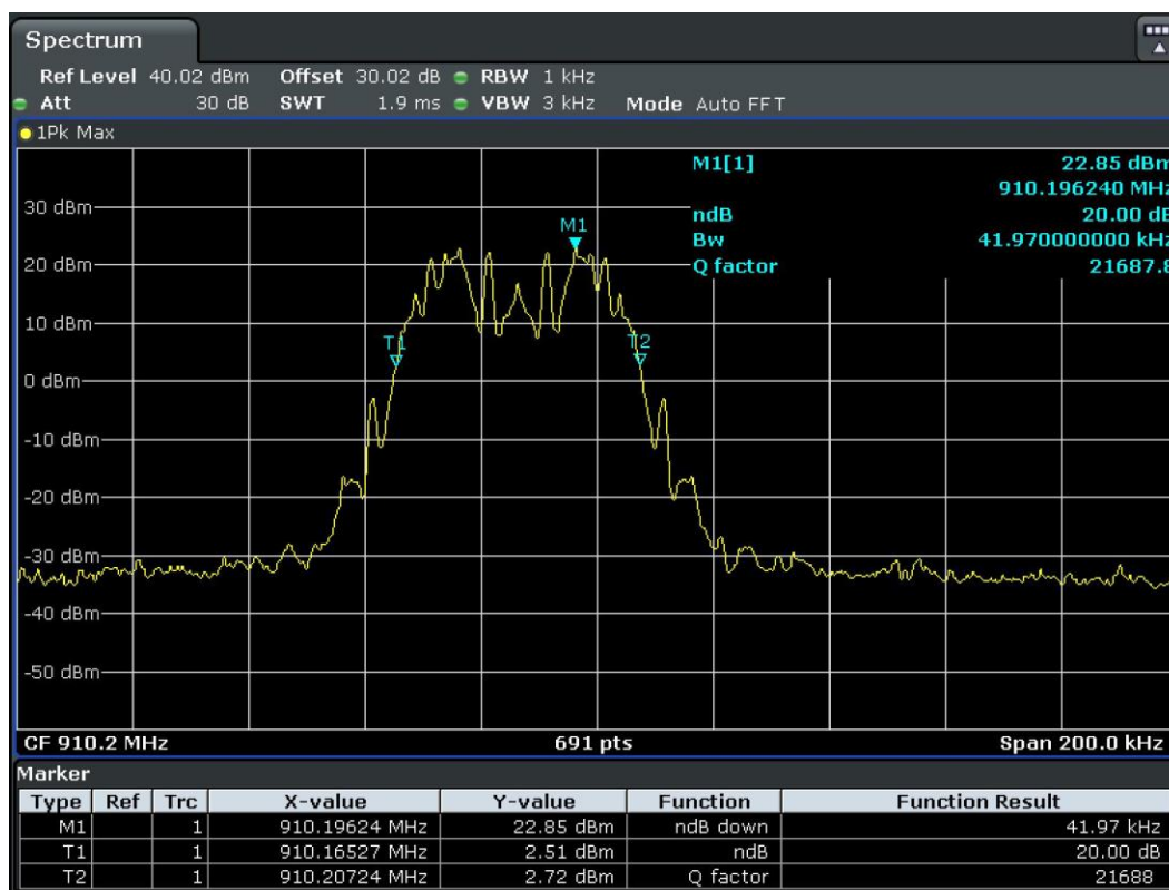
Figure 19. 20dB Bandwidth: Low Channel, 910.2 MHz, Antenna 1 Plot
