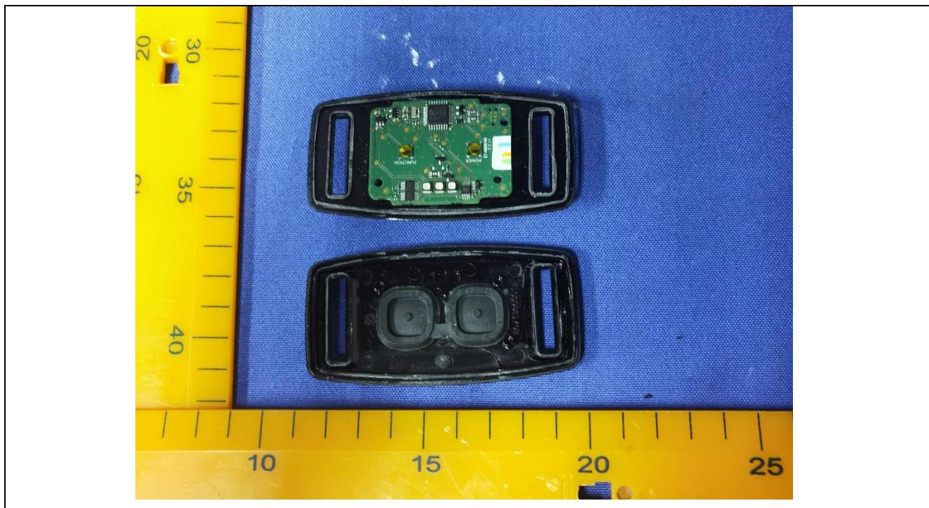
Details of: PCB view of alternative controller
