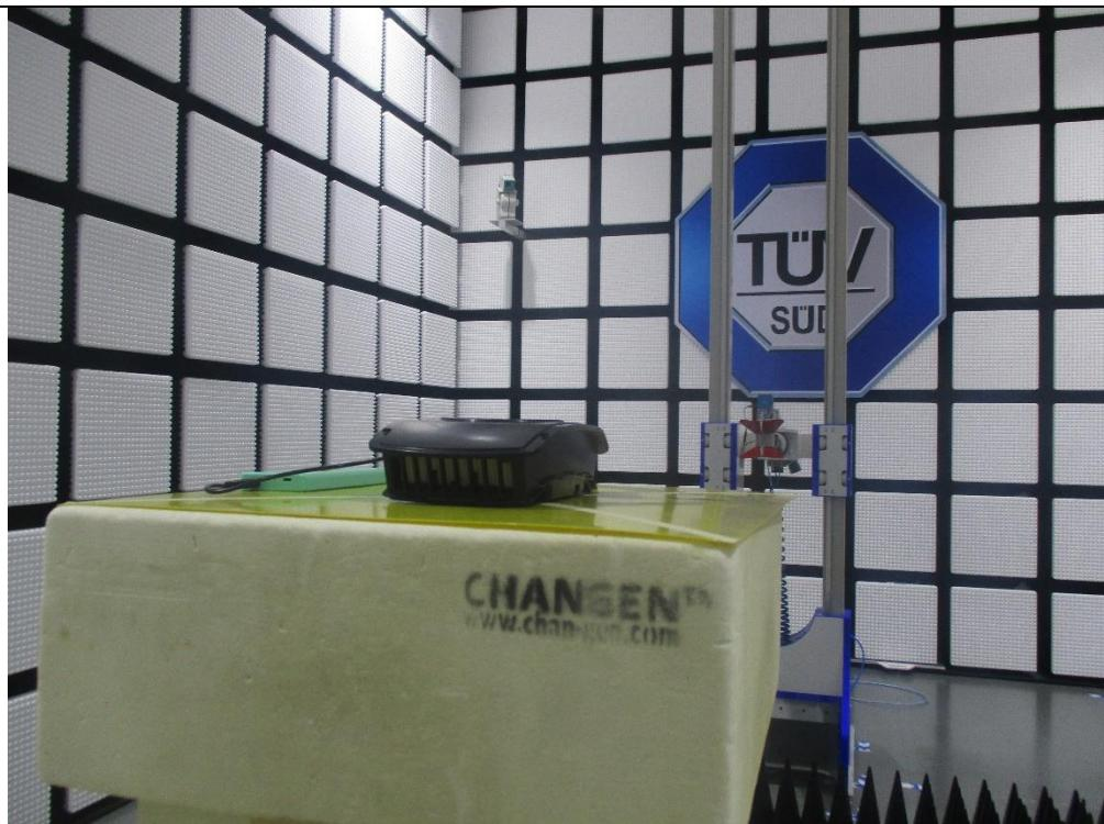
Radiated Emission test (Above 18000MHz)
