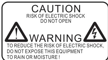
⑯ The lightning flash with arrowhead symbol within an equilateral triangle is intended to alert the user to presence of on-insulated hazard voltage within the product's enclosure that may be of sufficient magnitude to constitute a risk of electric shock.
