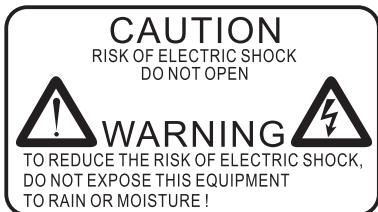
⑰ The lightning flash with arrowhead symbol within an equilateral triangle is intended to alert the user to presence of on-insulated hazard voltage within the product's enclosure that may be of sufficient magnitude to constitute a risk of electric shock.
