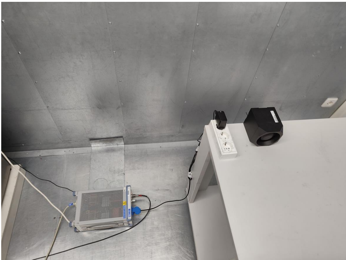
Figure 6: Conducted measurements on AC lines test setup
