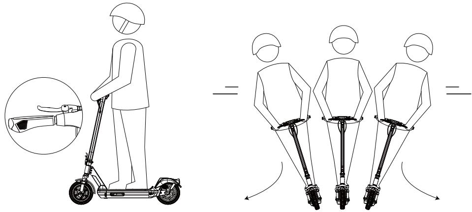
4. Release the accelerator and the kinetic energy recovery system initiates automatically to brake slowly; And squeeze the brake lever for a sudden brake.
