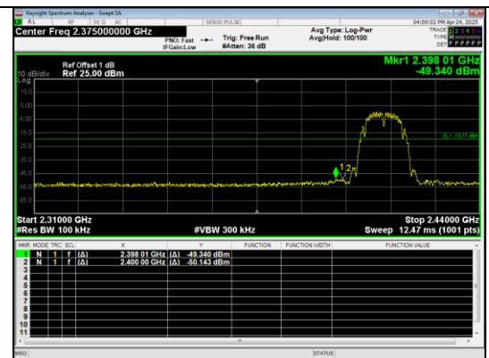
Out Of Band Emission IEEE 802.11b_Channel 1_20MHz_Antenna 2
