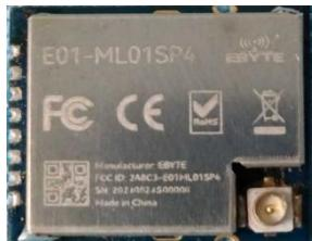
E01-ML01SP4 is a small-size SMD wireless transceiver module, operates at 2.4 GHz., with high data rate (Max 2Mbps) and SPI interface. The IPEX interface designed on the module is convenient to connect external antenna. Cost-effective and Batch production, which make the module suitable for various applications.
