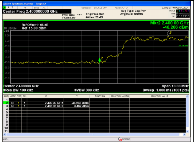
Out Of Band Emission(Left) \pi/4 DQPSK_2-DH5_Channel Hopping
