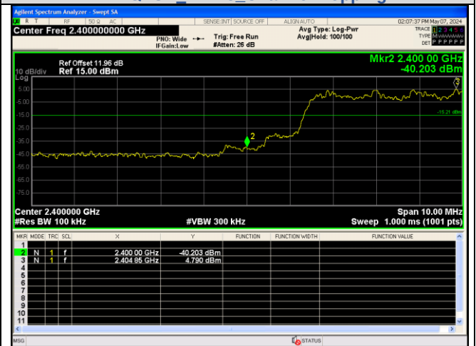
Out Of Band Emission(Left) \pi/4 DQPSK_2-DH5_Channel Hopping
