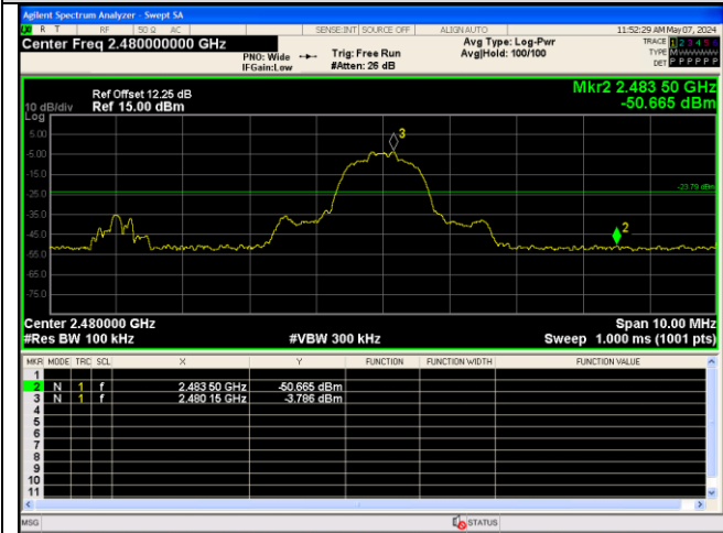
Out Of Band Emission 8DPSK_3-DH5_Channel 78
