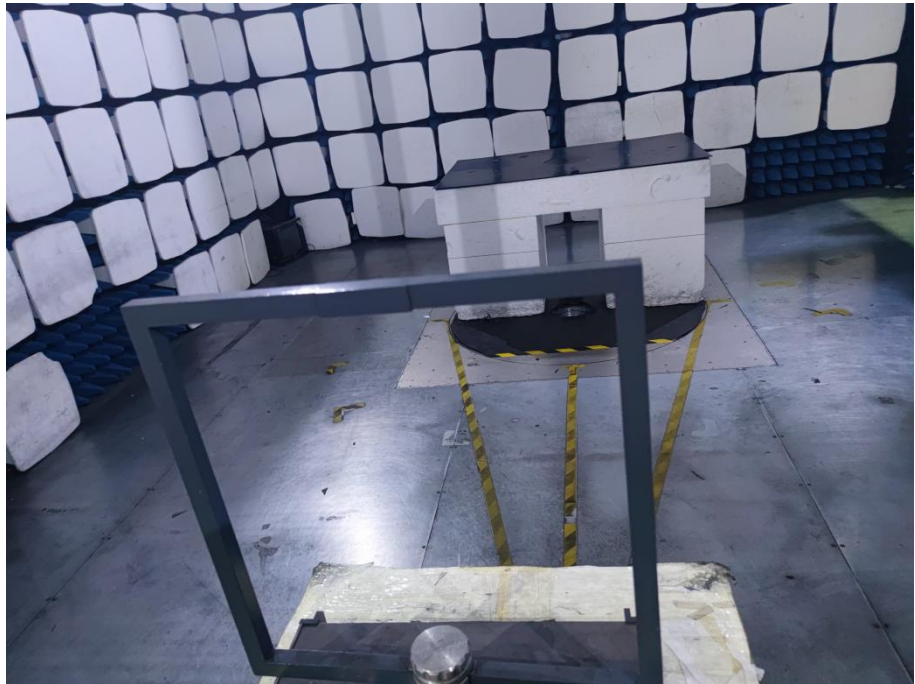
Radiation Emission Test Setup (Below 30MHz)
