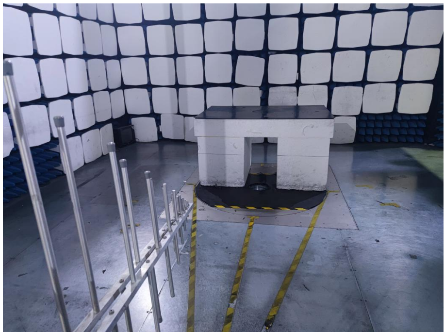
Radiation Emission Test Setup (30MHz to 1GHz)
