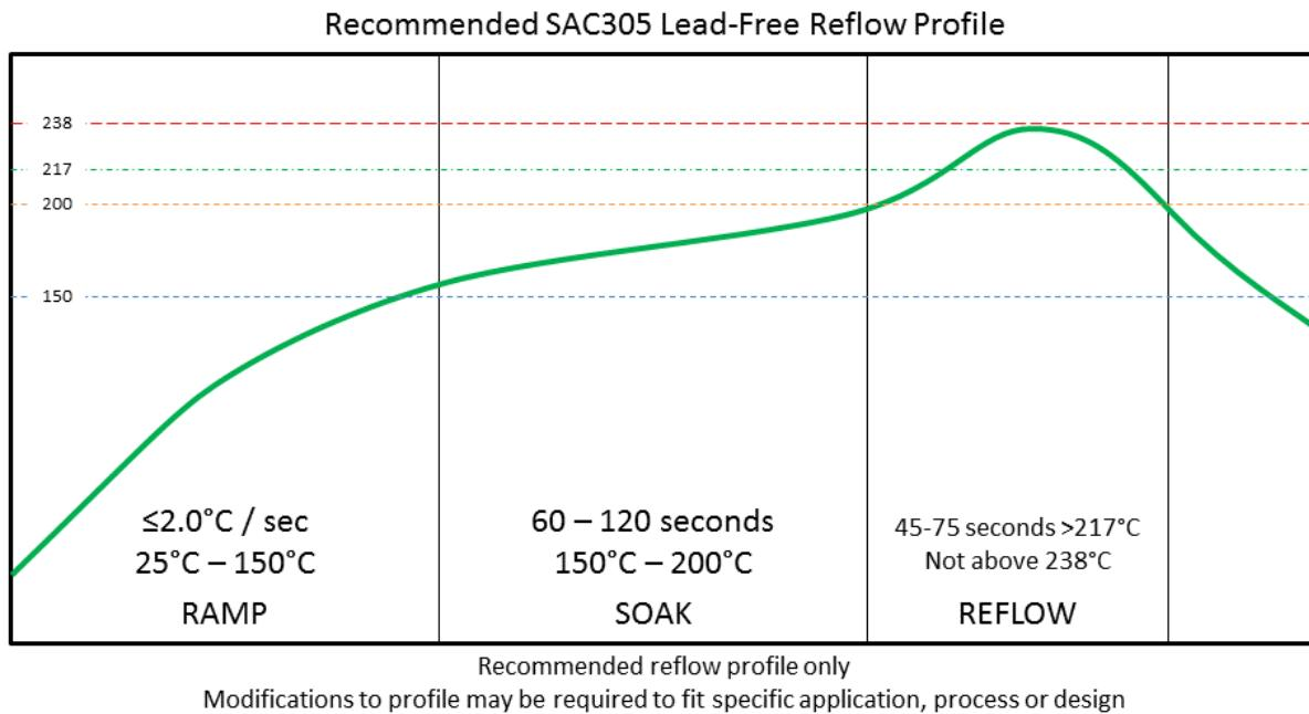
The device reflows during this cycle, and must not be reflowed upside down. Be careful not to jar the device while the solder is molten, as parts inside the device can be removed from their required locations.
