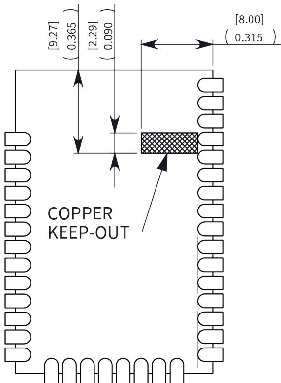
**Copper keepout for the XBee 3 Micro**
