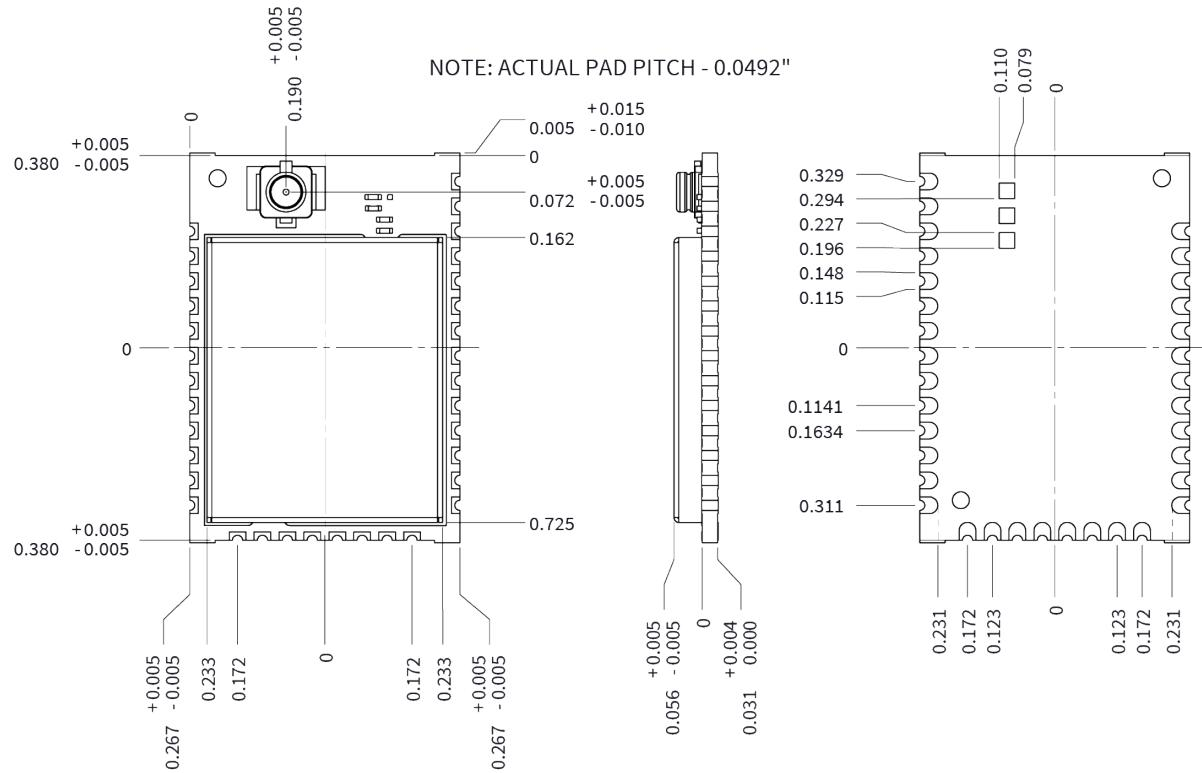
**XBee 3 micro (chip antenna)**
