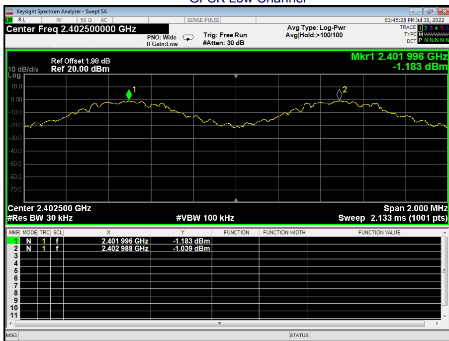
Test plots GFSK Low Channel
