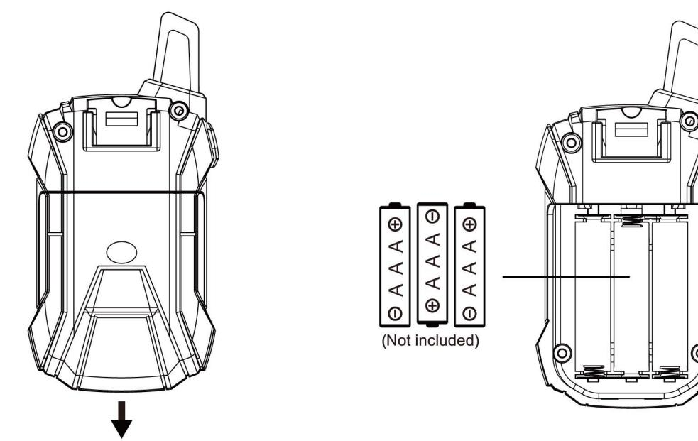
Press down on the back of panel of the unit and slide the battery cover off. (you may need to remove the belt clip for easier access).
