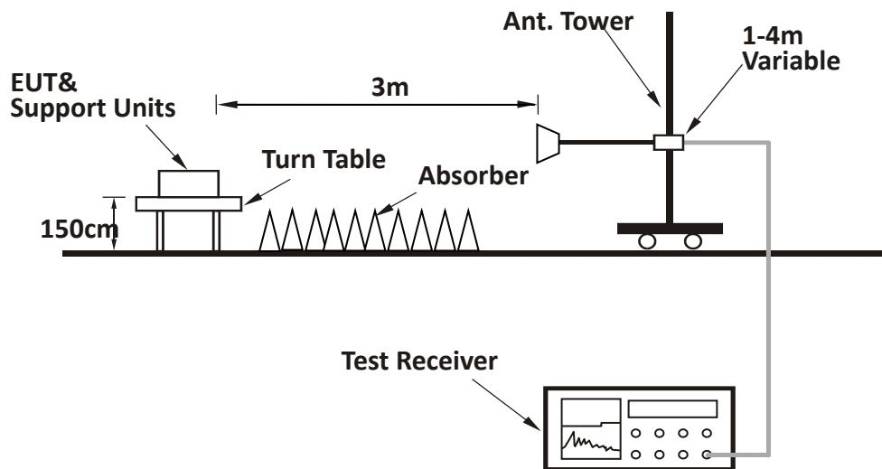
**TEST REPORT****3.4 Test Results of Radiated Emissions**
