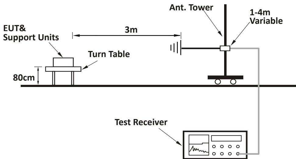
**TEST REPORT****For Radiated emission above 1GHz:**
