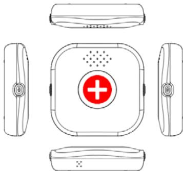
2、 Press left side battery check button within 1 second, device to say "battery ok". Front LED light green .If device to say "Please change battery" Front LED light will light red ,please replace new battery. If LED is not on, please recheck position of batteries.
