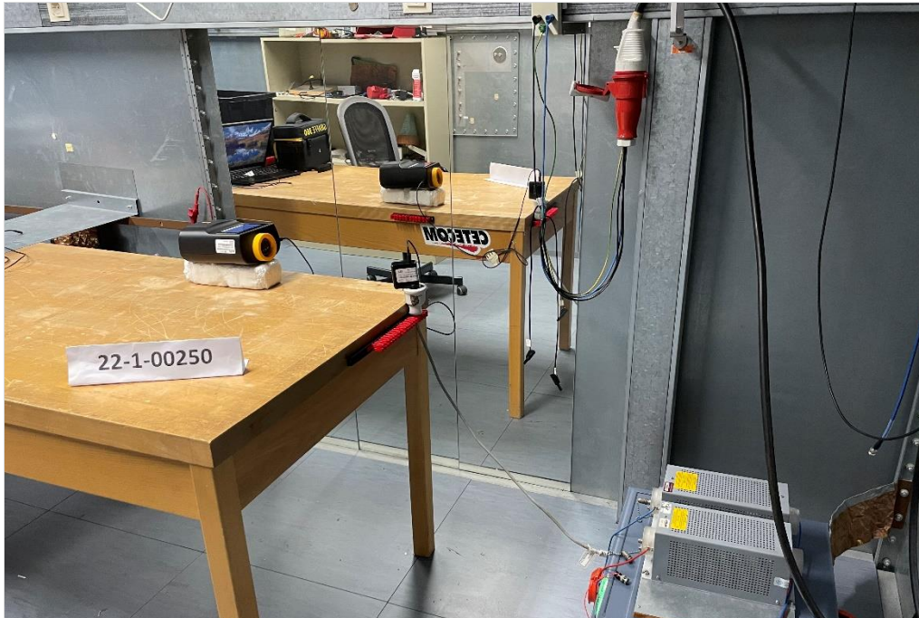
Photograph 11: EUT test setup for AC Conducted Emissions, overview
