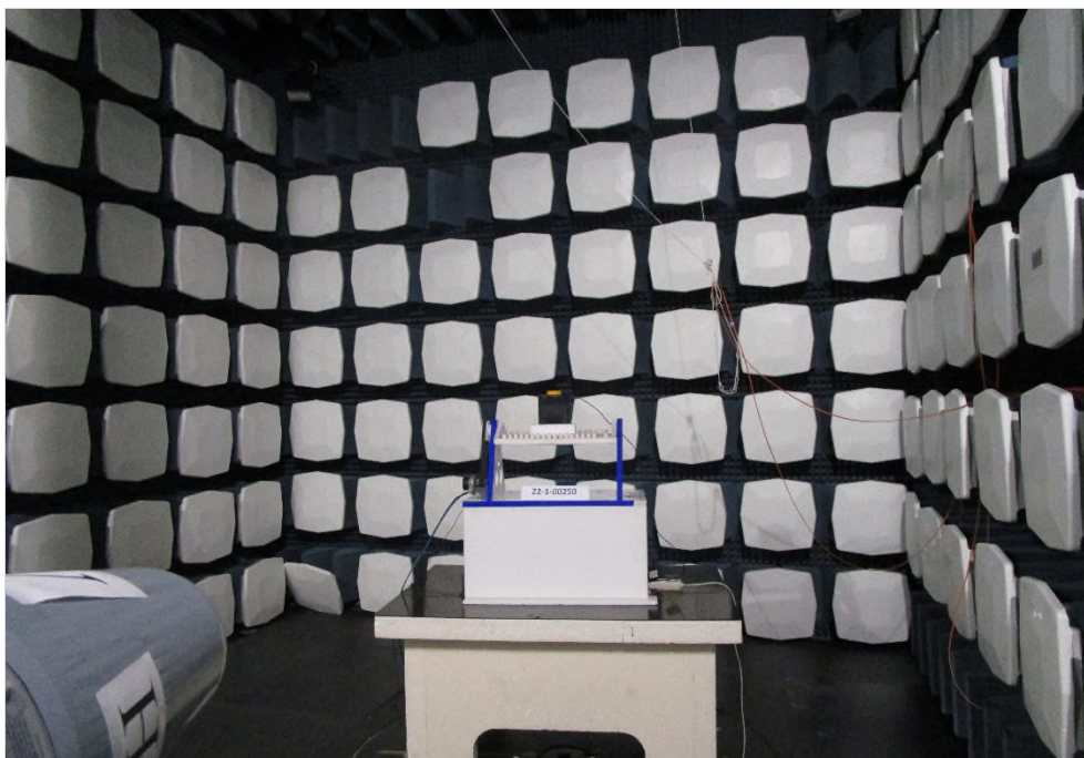
Photograph 10: EUT test setup in the fully anechoic chamber, overview_standing
