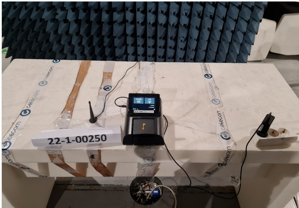
Photograph 3: H-Field test setup in the semi anechoic chamber, close up view_laying
