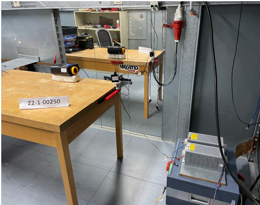
Photograph 11: EUT test setup for AC Conducted Emissions, overview
