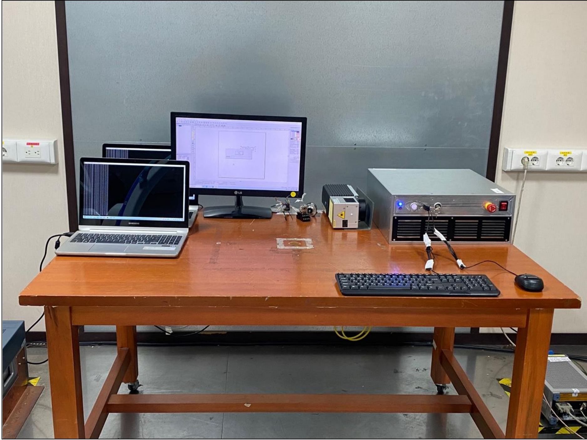
Continuous Conducted Emission at main _ Front
