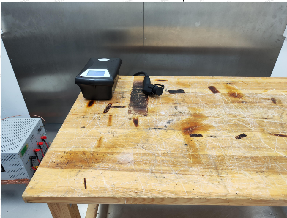
Photo of Radiation Emission Test (below 1GHz)
