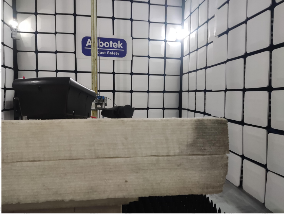
Photo of Radiation Emission Test (above 1GHz)
