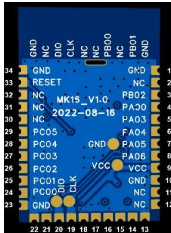
Figure 4: MK16 module pin-out (Rear View)
