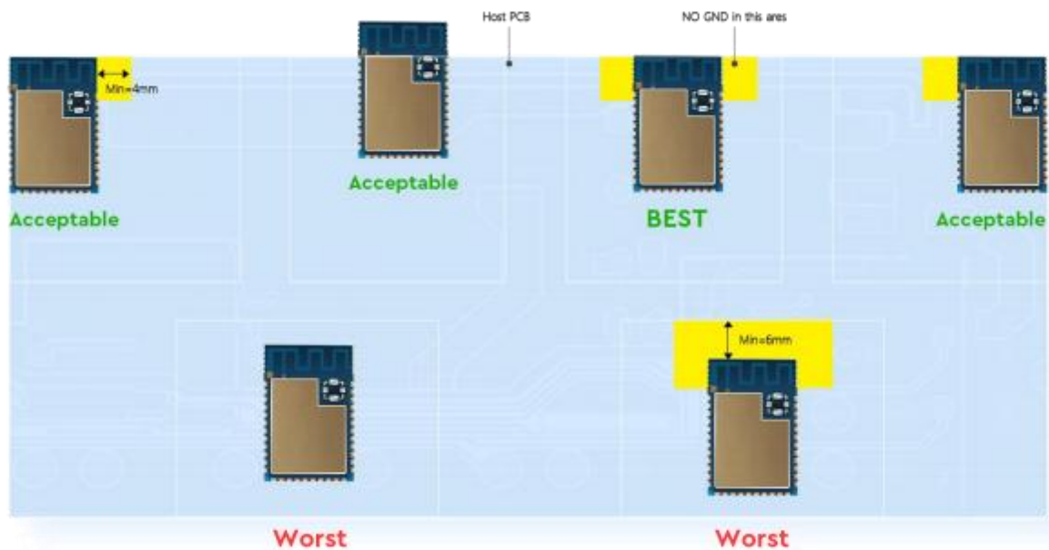
Figure 8: Recommended Module Mounting Examples
