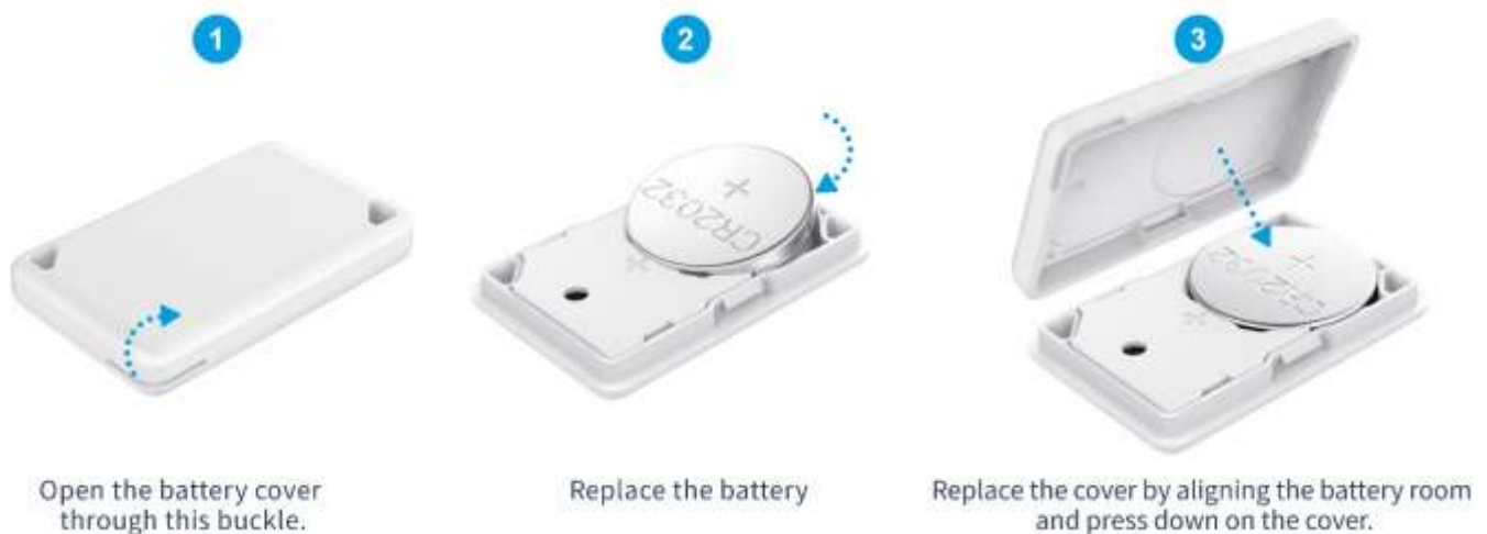
Figure 4: How to replace the battery of M4 Lite Tag?
