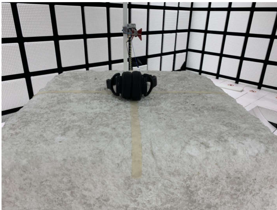
Radiated spurious emission Test Setup-2(Above 1GHz)
