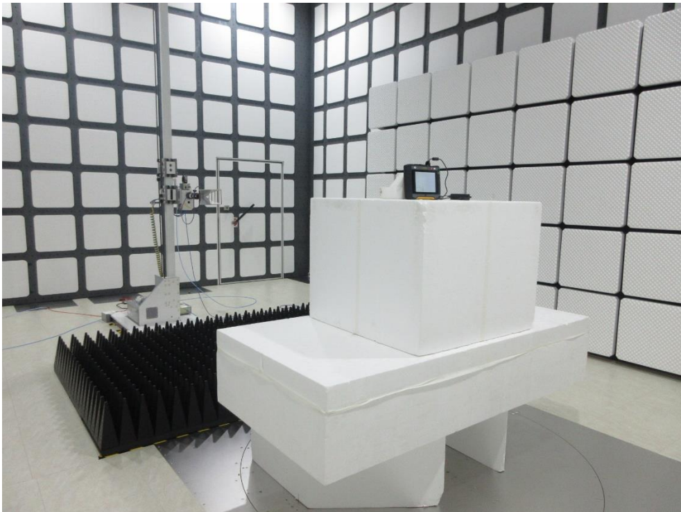
Description: Radiated Emission Test Setup for 1GHz~18GHz
