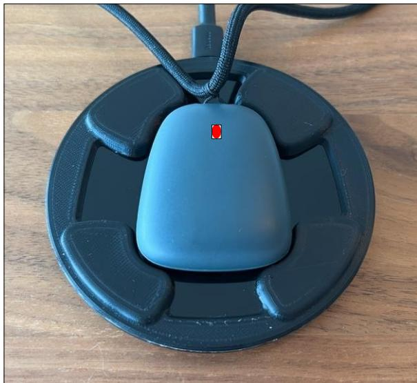
If the status indicator blinks red instead of “breathing” green after you have placed the wearable on the charger, the current device temperature is too high to charge the battery.
