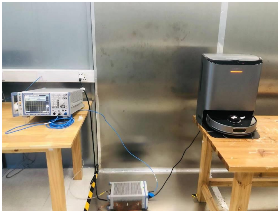
Photograph 3: Set-up photo for Conducted Emission
