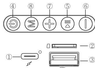
1.DC 5V slot: Use the standard USB TYPE-C charging cable for power charging.
